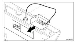
The control module is fitted in the tower after the cover plate has been unscrewed from the ceiling.
